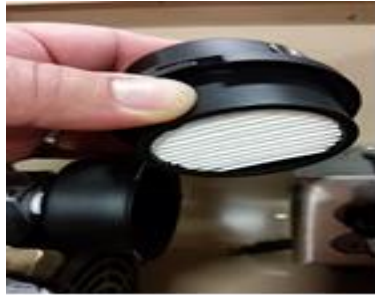
Remove top of filter housing clean or replace
