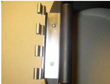
Attach provided Hinge to Hopper Top Section using two 1" long bolts. Place bolts down through hinge and through hopper, then attach washer and lock nut on each screw from inside the hopper.
