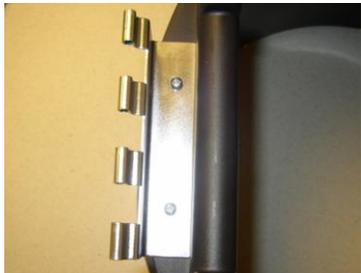
Attach provided Hinge to Hopper Top Section using two 1" long bolts. Place bolts down through hinge and through hopper, then attach washer and lock nut on each screw from inside the hopper.
