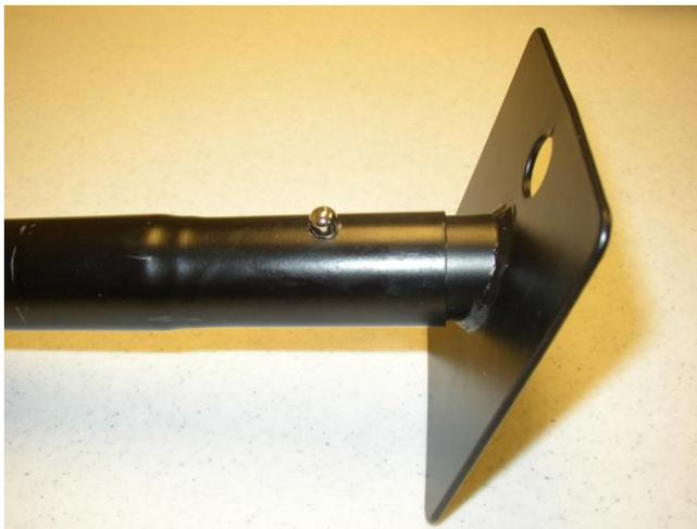
If using the provided Metal Feeder Feet, we recommend drilling one hole on the smaller end of a leg section for the pop-up clips. Drill a 5/16" hole centered exactly 1 1/4" up from the end. Attach feeder feet, then attach leg by sliding it up the square receiver.
