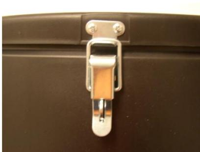
Attach the Strike to the Hopper Lid and Catch to the Hopper Top using four 1/2" long screws as shown. Inside the Hopper, place a washer and lock-nut on each screw.
