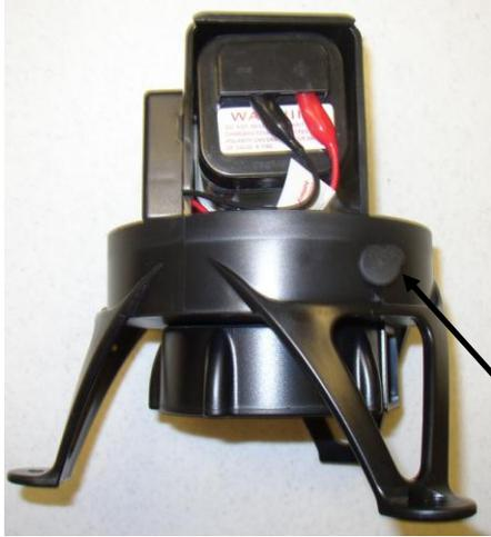
Go ahead and insert the 6 volt battery into the feeder housing. Use alligator clips to attach as shown in picture. Go ahead and program the current time and feeder timer. Note: Timer should be automatically preset to feed two times a day. Change as needed.
