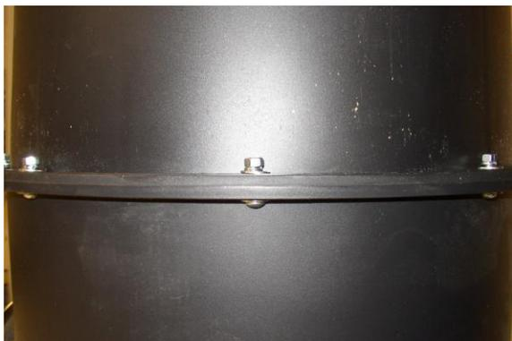
Place Hopper Bottom Section on Hopper Top Section as shown. For each of the nine holes, insert provided 1" long bolt through a washer, the Hopper Bottom Junction Ring, another washer, lock-washer and onto the nut as shown. Use a wrench to tighten each of the nuts.
