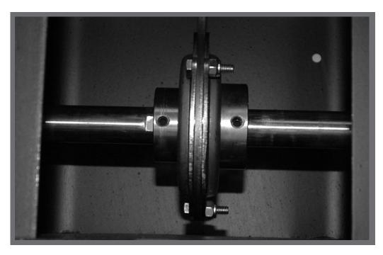
New SS Excentric is precision machined and has two set screws with a locking snap ring. Most importantly, the center bearing is balanced in the middle of the crankshaft to equalize the workload for less bearing failure. All three bearings are inside the compressor and sealed. With today's advanced bearing technology, you do not need to climb 20' in the air to grease bearings every year.
